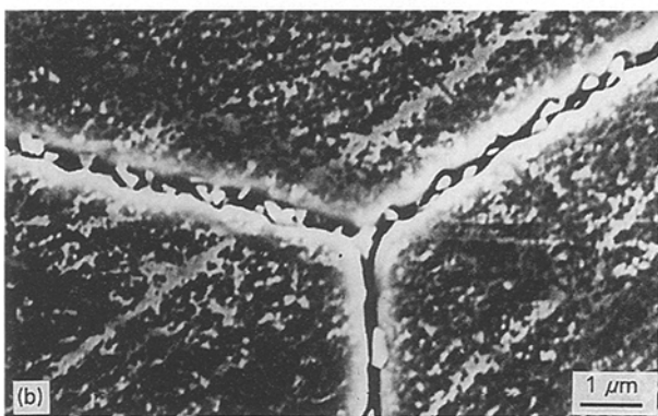
Figure 3 Effect of time and temperature of ageing on the degree of sensitization of 304SS material.
